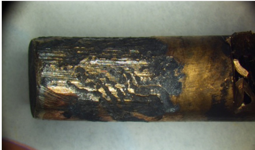
Arcing caused by the poor electrical connection.
