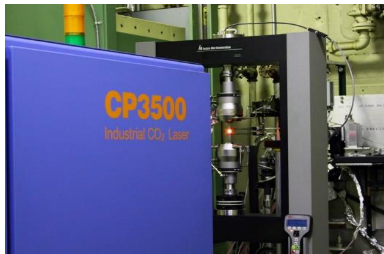
Laser high heat flux creep rupture test rig
