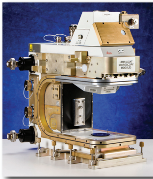
A modified Leica RXA research imaging light microscope with powerful laser-diagnostic hardware and interfaces.
