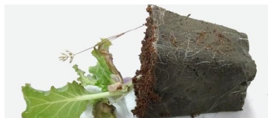
Figure 10: Root Ball. Root ball of plant grown in lunar regolith simulant, removed from its pot.
