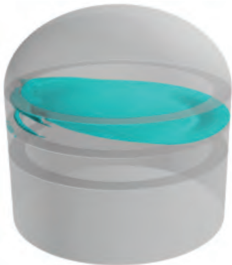
VoF method CFD simulation of propellant slosh within a propellant tank with ring baffles.
