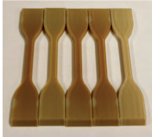
Four UV-exposed Ultem samples, control sample on right.
