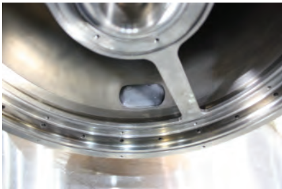
Wireless sensor (black) molded onto the wall of the Distillation Assembly.
