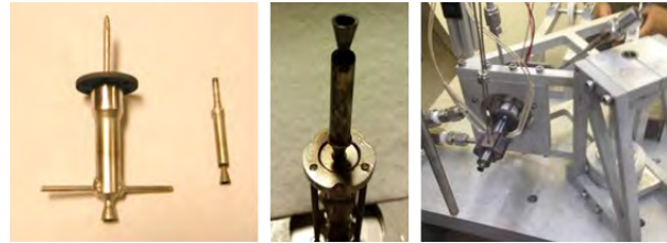
Left: PPI 1-N and 100-mN thruster reactors. Center: 100-mN thruster post hot-fire test. Right: 1-N thruster in Cell A.
