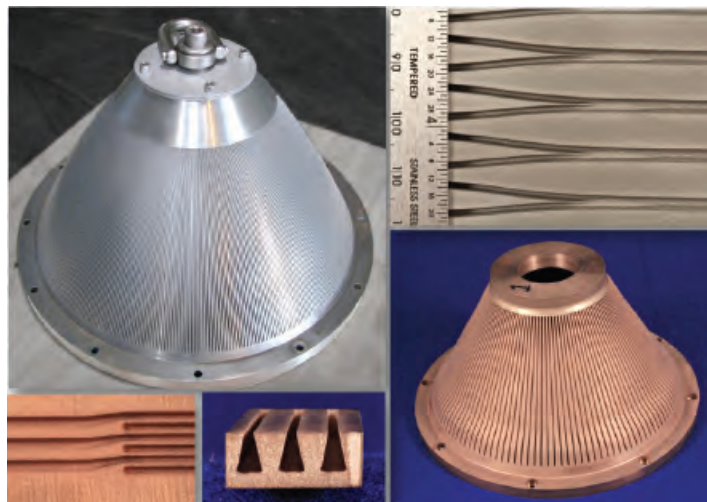
Examples of advanced engine design concepts manufactured using a variety of metals and machined using the novel water jet milling process.
