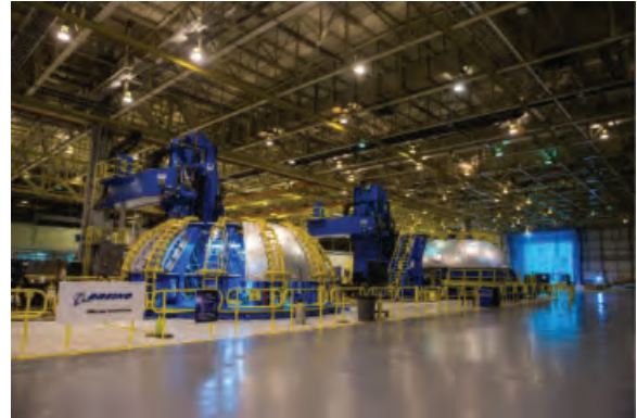
FSW of SLS CS domes on robotic weld tools at Michoud Assembly Facility.
