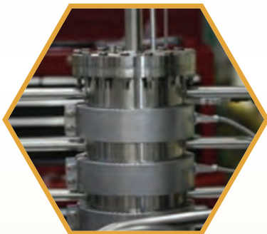
Reverse Water-Gas Shift Reactor with band heaters and integrated thermocouples
