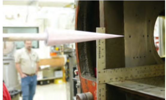
A model prepared with pressure-sensitive paint waiting for a wind tunnel test.
