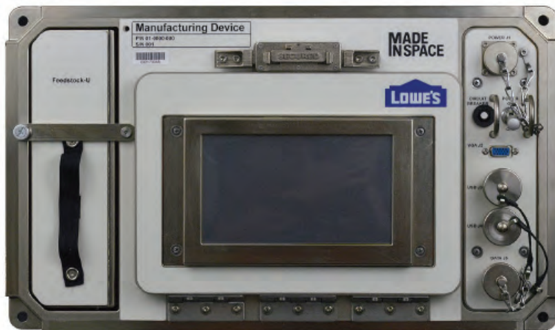
The ISS flight demonstration additive manufacturing device provided by MIS.
