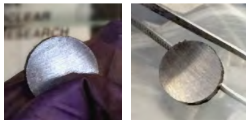
Sample NASA-SPS-1800C-002 after removal of Grafoil on ends. (26.0579 g)
