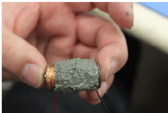
Install heater, wire-side up, on putty-coated side of cell. Apply new coat of putty to fill in any cracks.
