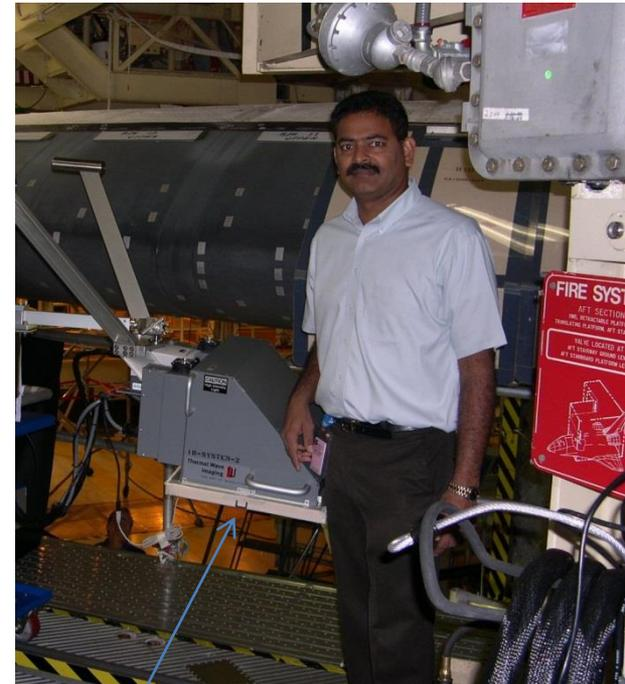
Flash IR Hood attached to Strong Arm that is attached to a cart on rails. Worked as a project engineer to develop and implement IR thermography Inspection of Orbiter wing leading edge at Kennedy Space Center
