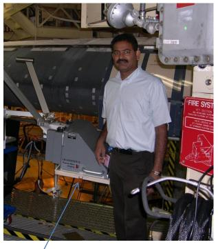
Flash IR Hood attached to Strong Arm that is attached to a cart on rails. Worked as a project engineer to develop and implement IR thermography Inspection of Orbiter wing leading edge at Kennedy Space Center
