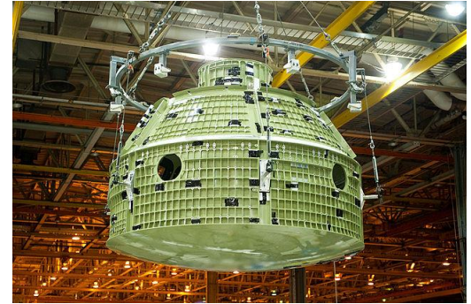
EFT-1 Orion after final weld on June 22, 2012.
