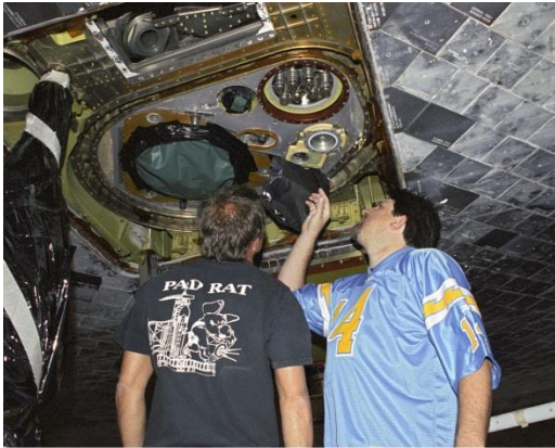
NASA Dryden Flight Research Center Photo Collection http://www.dfrc.nasa.gov/Gallery/Photo/index.html NASA Photo: ECI05-0166-20 Date: August 12, 2005 Photo By: Tony Landis Technicians inspect external tank attachment fittings on the Space Shuttle Discovery as part of it's post-flight processing at NASA DFR.
