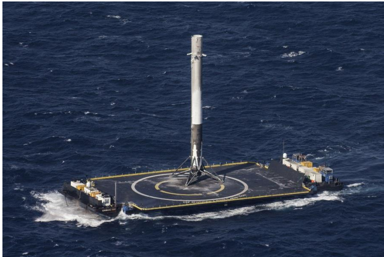
Falcon 9 first stage on an ASDS barge after the first successful landing at sea, CRS-8 Mission. April 2016
