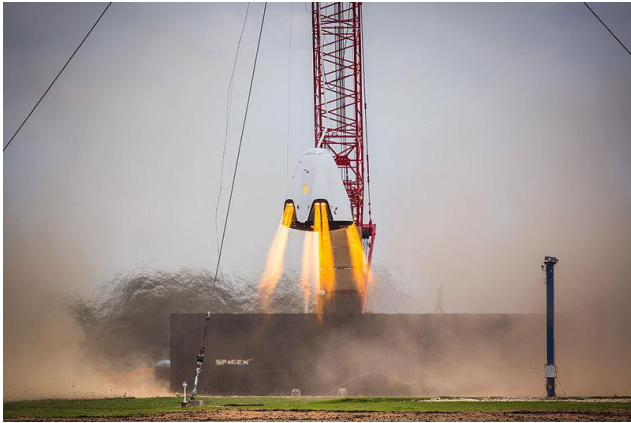
Dragon 2 spacecraft conducting a propulsive hover test, Nov. 2015
