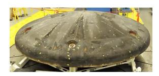
EFT-1 Orion heat shield 5 meter diameter
