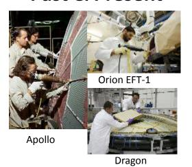
Labor intensive Heat Shield Manufacturing
