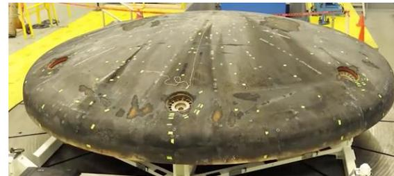
EFT-1 Orion heat shield
