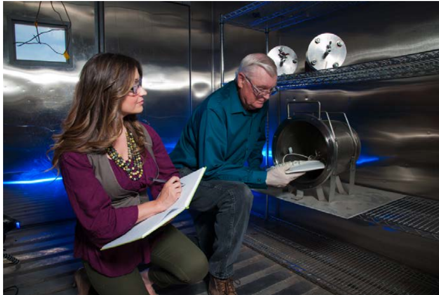
Figure 1. Sample loading. Materials or assembled articles are loaded into sealed, certified-clean containers and thermal conditioning for 72 ( \pm 1 ) hr at 50 ( \pm 4 ) °C (122 ( \pm 7 ) °F) prior to performing analysis of the test atmosphere.
