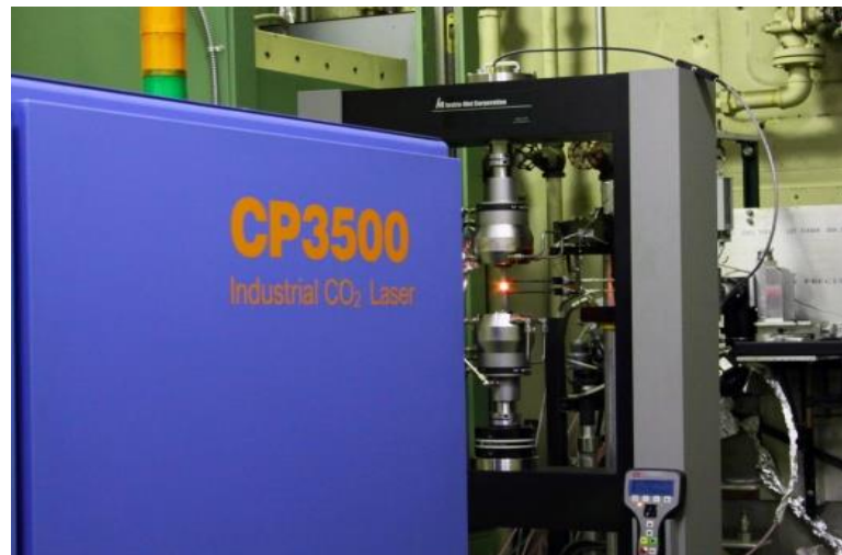
High heat flux combustor rig
