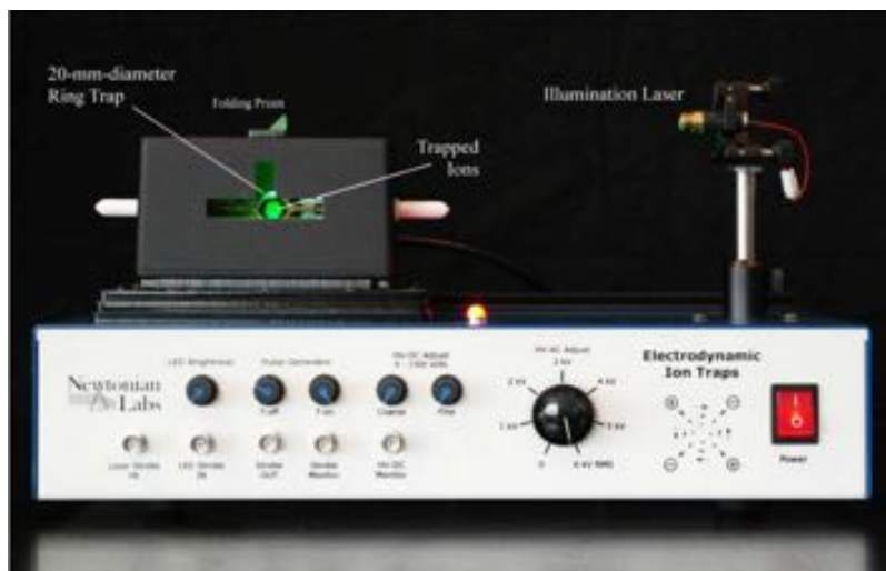
Figure 158. Elements of ion trap used in tests (from Newtonian Labs).
