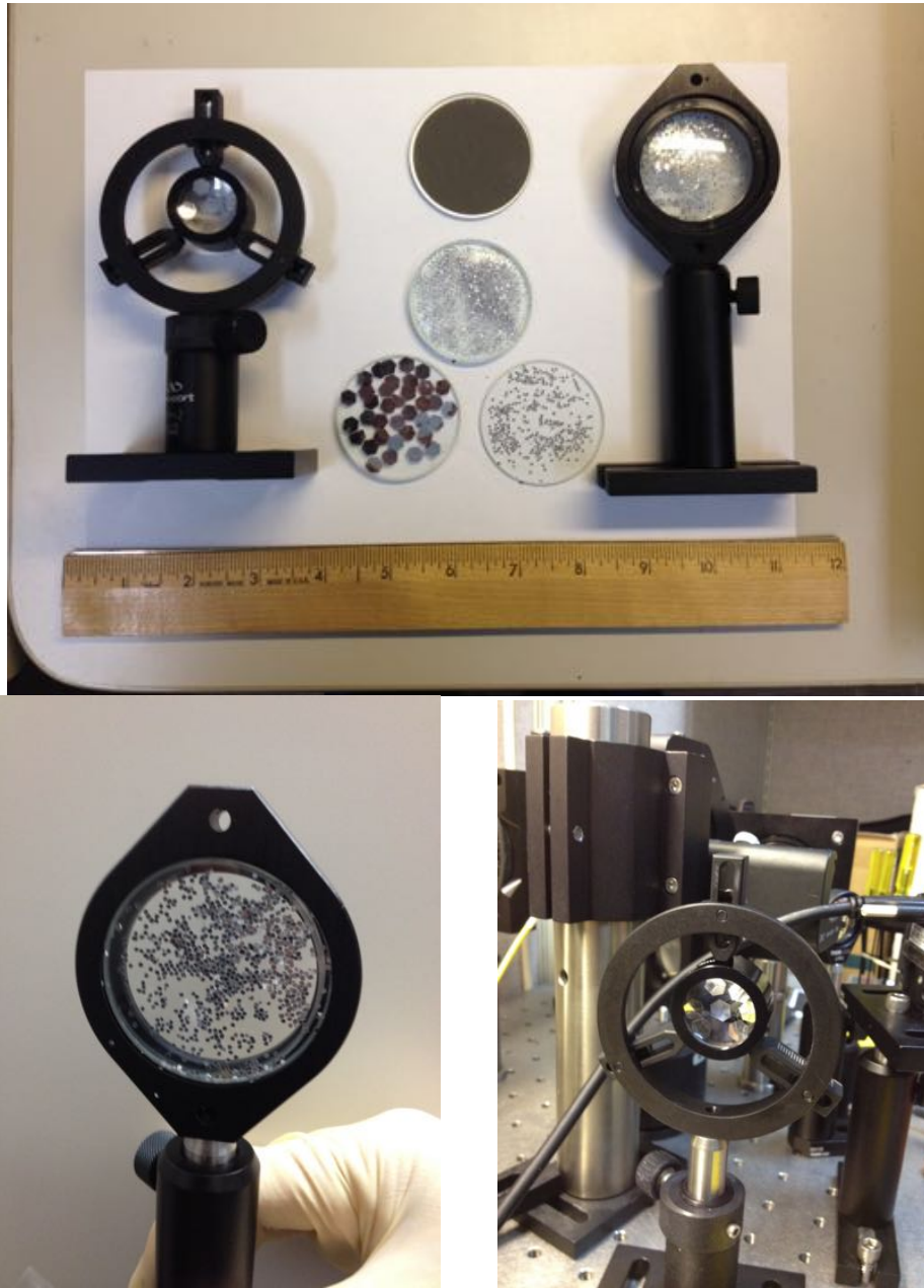
Figure 93. Different granular lenses used in the experiments.
