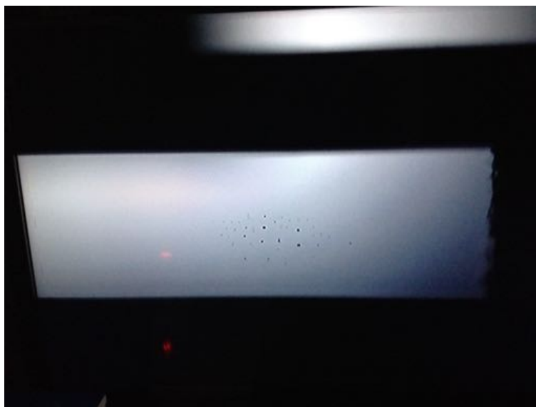
Figure 161. Photo of levitated cloud of silver coated hollow glass microspheres (100 micron diameter).
