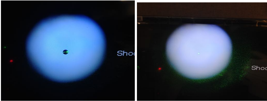
Figure 168. Photo of levitated grain of silver coated hollow glass microsphere (100 micron diameter).
