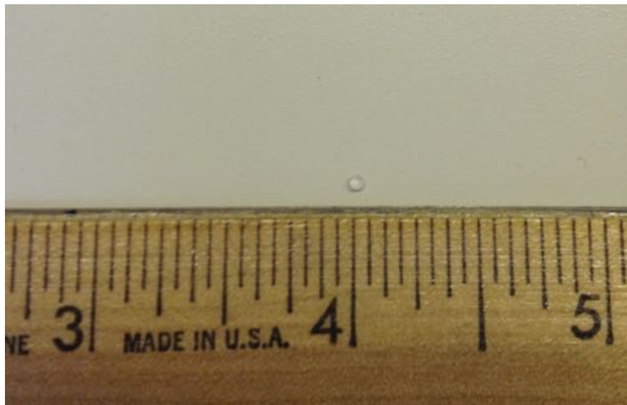
Figure 30. 0.3 mm hemispherical grain.
