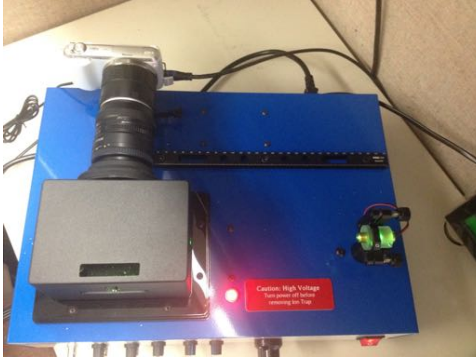
Figure 160. Top view of ion trap chassis, showing camera with zooming lens, illuminated laser, and trap.
