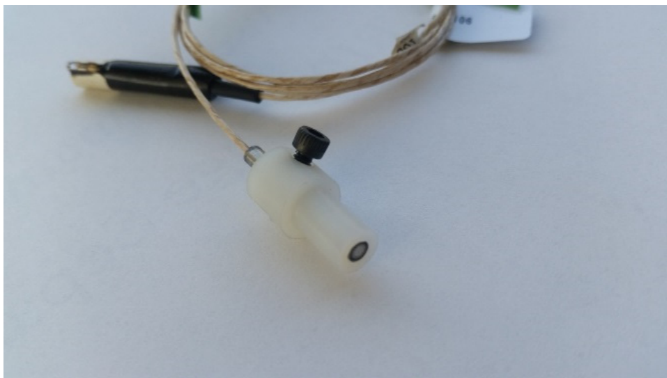
Figure 4.—In-duct Array Kulite® Sensor Insert.
