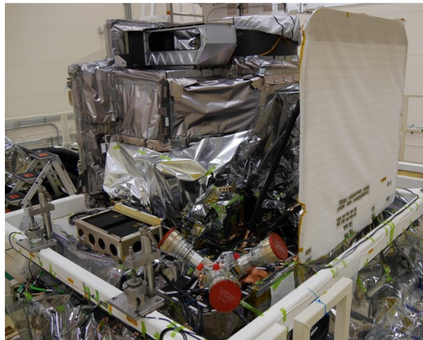
Fig. 16. EPP flight configuration of GOES-R (prior to final thermal blanket installation)
