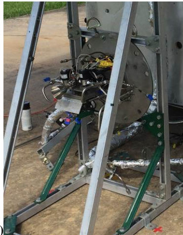
Figure 6. a) CryoCart test article with vacuum pipe apparatus for hot-fire testing. b) 28 lbf-vac RCE with coil-on-plug igniter mounted on vacuum pipe interface plate, c) 28 lbf-vac thruster mounted on ambient checkout test stand.
