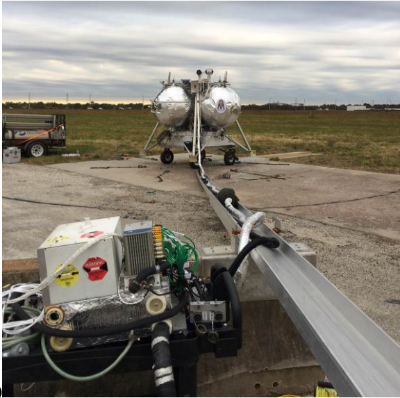
a) ICPTA sea-level hot-fire configuration with Plum Brook 50 ft avionics harness. b) Hot-fire demonstration with main engine and RCS simultaneous operation with coil-on-plug igniters
