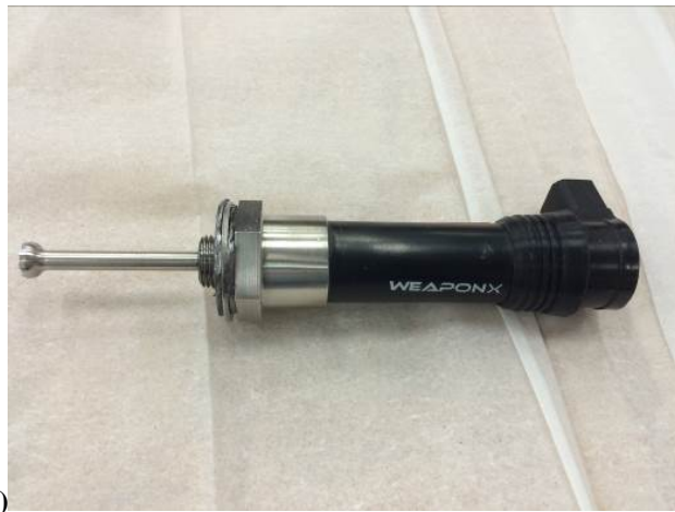
a) b) Figure 3: a): Conventional spark plug with external coil and high-voltage cable used during sea-level testing. b): Coil-on-plug spark plug system with high voltage cable eliminated, used for simulated altitude testing
