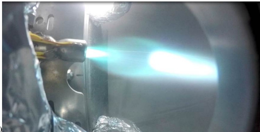
Figure 7. a) 281bf-vac RCE and b) main engine igniter testing in a vacuum conditions in CryoCart Vacuum pipe using coil-on-plug igniters.
