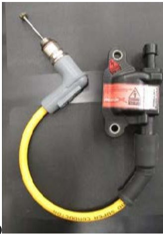
a) b) Figure 3: a): Conventional spark plug with external coil and high-voltage cable used during sea-level testing. b): Coil-on-plug spark plug system with high voltage cable eliminated, used for simulated altitude testing
