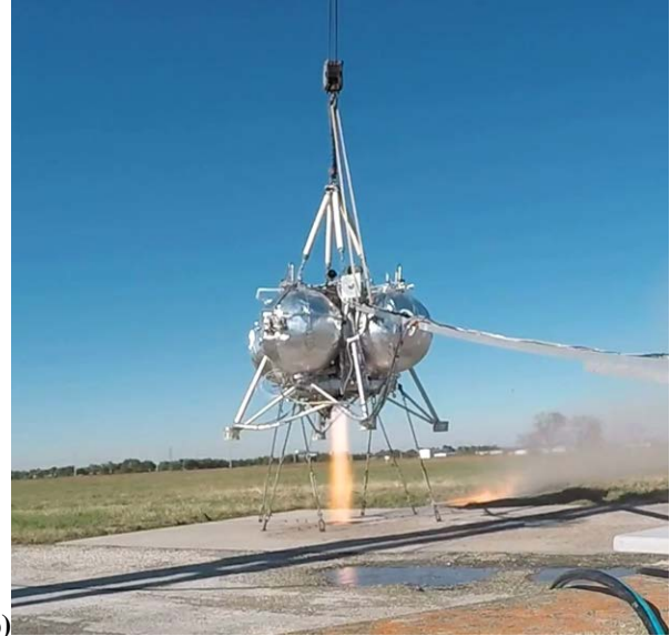
a) ICPTA sea-level hot-fire configuration with Plum Brook 50 ft avionics harness. b) Hot-fire demonstration with main engine and RCS simultaneous operation with coil-on-plug igniters
