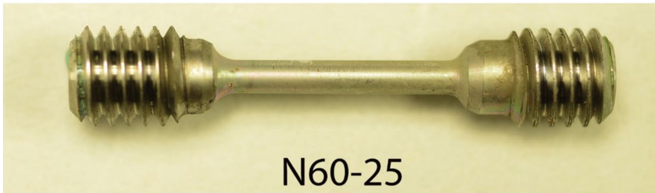
Figure 15. Metallographic and overall views of Nitinol 60 stressed to 50 ksi after a year-long exposure to sulfuric acid-based pretreat.
