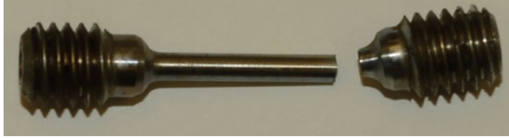
Sample N60-27-SABP-50: Stressed to 50 ksi, exposed for 1 year in sulfuric acid-based pretreat, and tensile tested to failure (153.2 ksi UTS)
