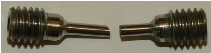
Sample N60-8-PABP-50: Stressed to 50 ksi, exposed for 1 year in phosphoric acid-based pretreat, and tensile tested to failure (176.1 ksi UTS)
