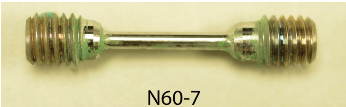
Figure 17. Metallographic and overall views of Nitinol 60 stressed to 50 ksi after a year-long exposure to phosphoric acid-based pretreat.
