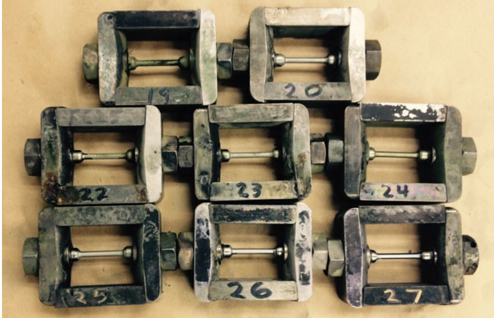
Figure 10. Nitinol 60 specimens after a year-long exposure to sulfuric acid-based pretreat.
