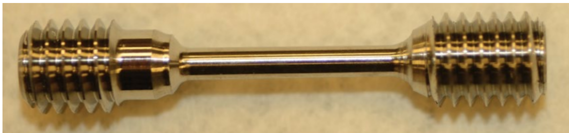
Figure 3. Photograph of Nitinol 60 round tensile specimen.
