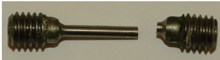
Sample N60-17-PABB-50: Stressed to 50 ksi, exposed for 1 year in phosphoric acid-based brine, and tensile tested to failure (152.4 ksi UTS)
