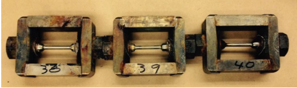
Figure 14. Nitinol 60 specimens after a year-long exposure to 3.5% NaCl alternate immersion per ASTM G44.
