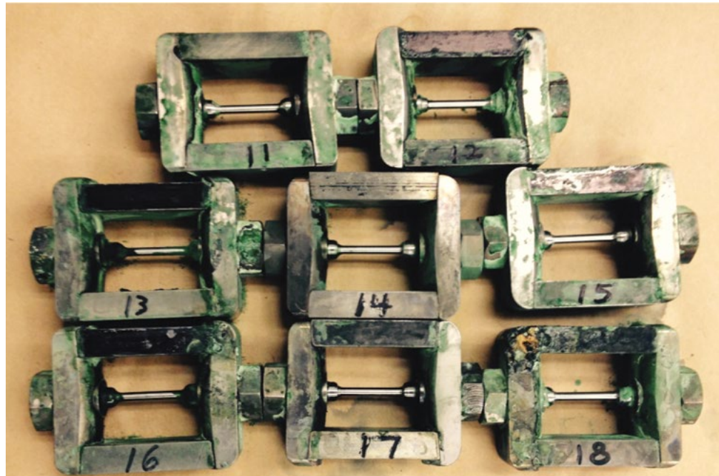
Figure 13. Nitinol 60 specimens after a year-long exposure to phosphoric acid-based brine.
