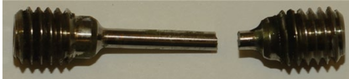
Sample N60-36-SABB-50: Stressed to 50 ksi, exposed for 1 year in sulfuric acid-based brine, and tensile tested to failure (152 ksi UTS)
