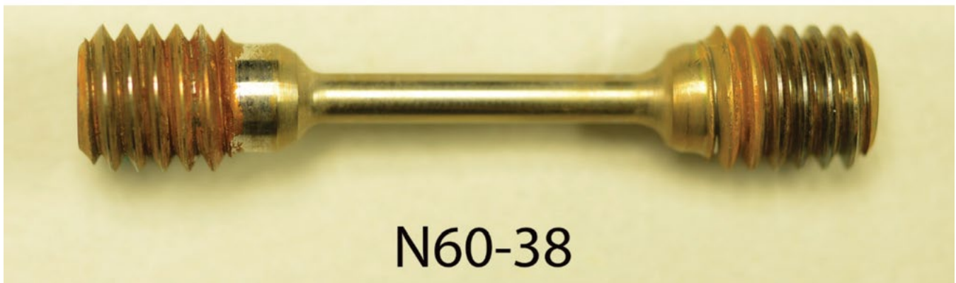
Figure 19. Metallographic and overall views of a Nitinol 60 specimen after exposure to 3.5% NaCl alternate immersion (365 days at 25 ksi and 32 days at 75 ksi).
