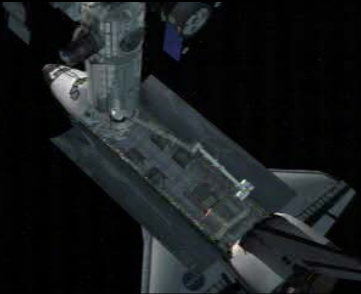
Airlock Installation Installed using the SSRMS
