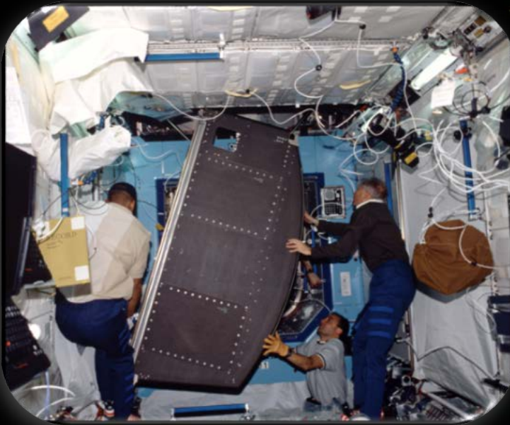
Rack Installation in LAB
