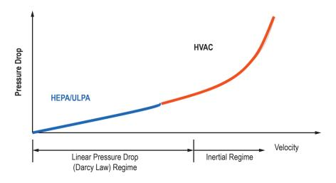
Figure 5. Influence of flow velocity on filter pressure drop. (© R. Vijayakumar. Used with permission.)
