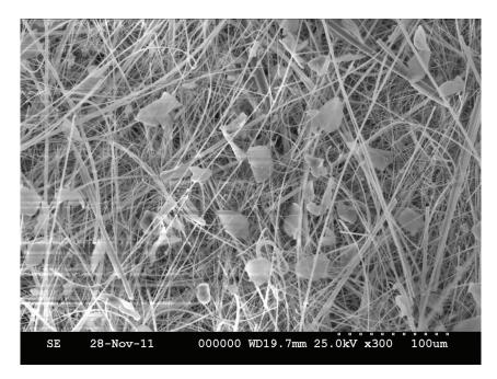
Figure 2. A SEM micrograph of ISS BFE media.
