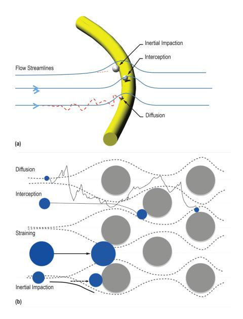
Figure 1. Particle-capturing mechanisms on (a) a single fiber and (b) fiber network. (© R. Vijayakumar. *Used with permission.*)
