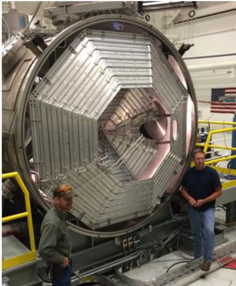
Figure 19. Iodine beam dump installed at chamber end showing backside, refrigerant tubing.
