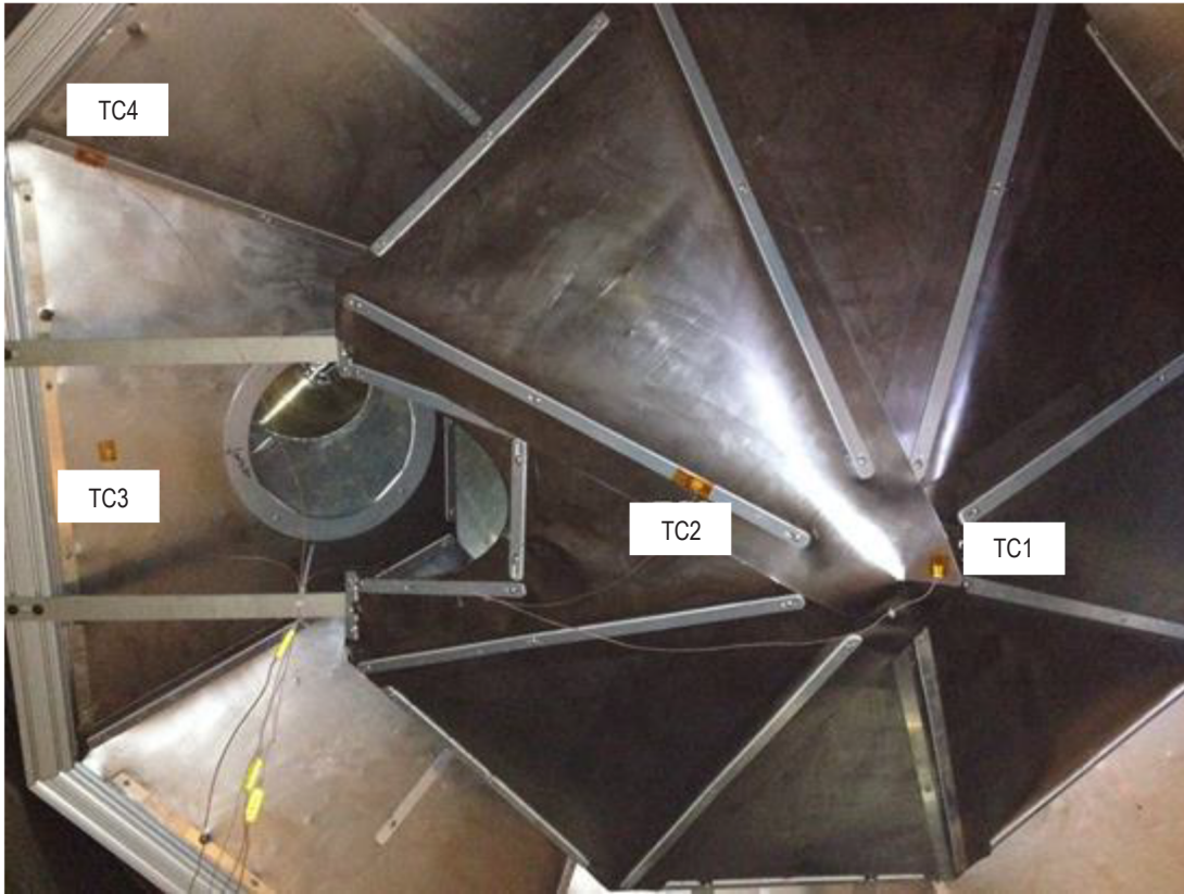
Figure 17. Beam dump image showing the location of four TCs used to measure the temperature at these locations as a function of time during one IBD cooldown cycle.
