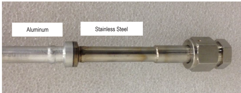
Figure 9. Aluminum (left part) to stainless steel (right part) explosively welded transition joint.
