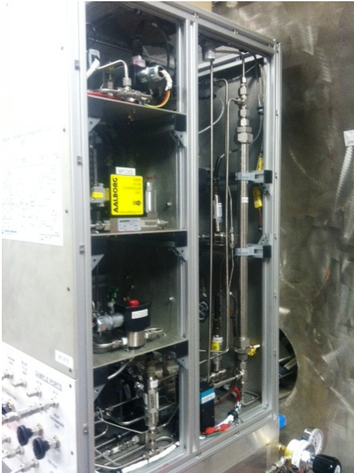
Sabatier Carbon Dioxide Reduction Assembly (CRA)
