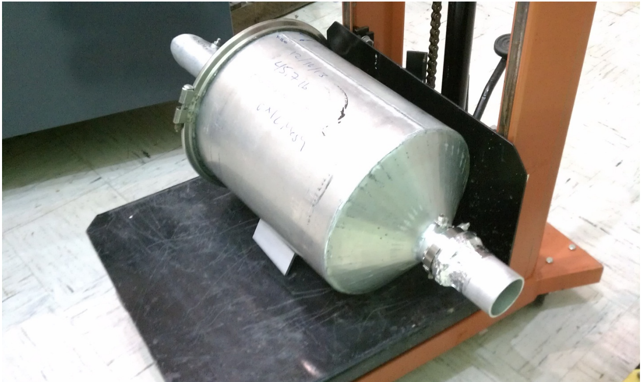
TCCS Low-flow Fixed Bed (LFB). NOTE: the LFB was not used after the Phase 4 evaluation showed that the ACFB would provide the required contaminant removal for Phases 5 and 6
