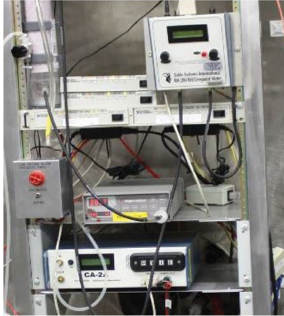
Figure 9. Major constituent analysis instrument array.
