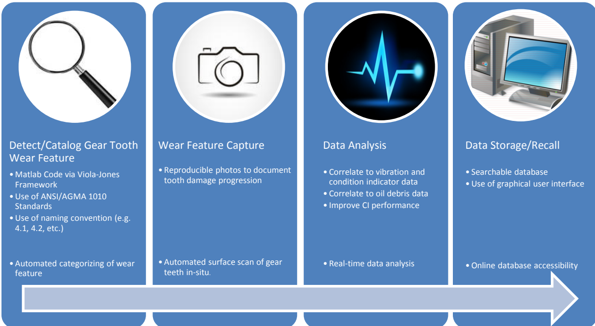
Figure 2.—Notional framework to analyze gear tooth wear.
