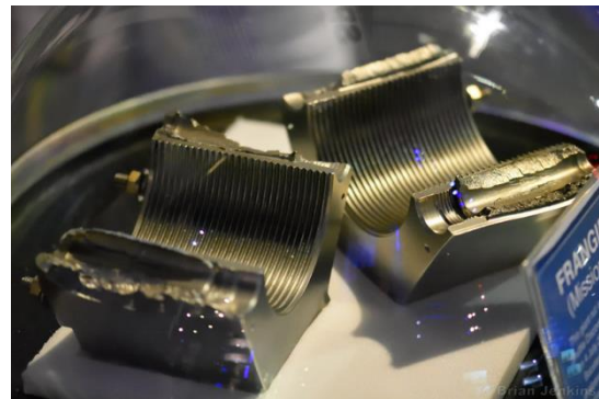
Figure 4 Frangible Nut after pyrotechnic severance Photo credit: NASA
