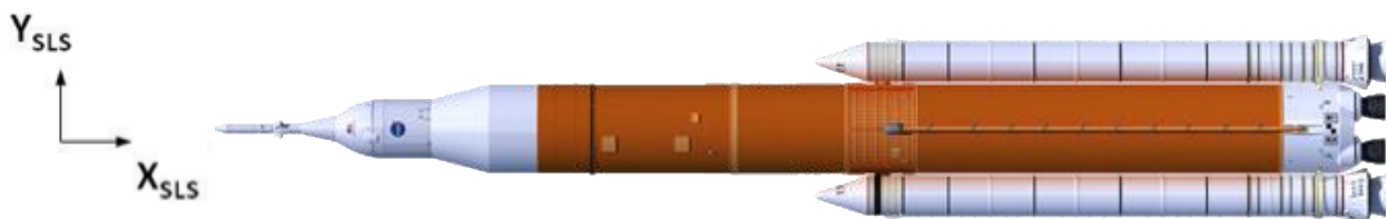
Figure 3-3. SLS Vehicle Coordinate System
