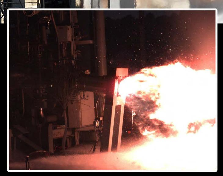
Hot-fire testing has demonstrated parts manufactured with this technique can survive and perform well in the relevant environments for liquid rocket propulsion systems.
