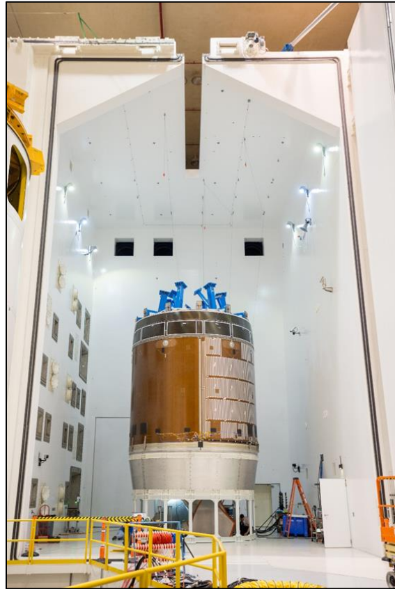
Figure 8. E-STA in RATF Reverberation Chamber.
