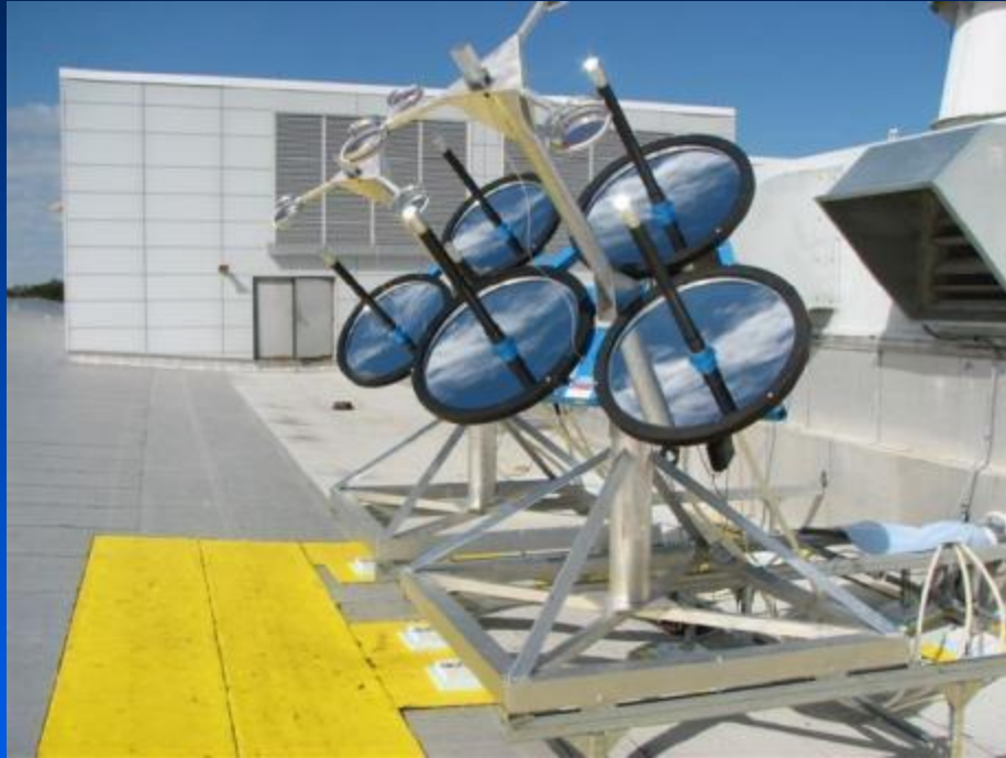
2 m 2 of collectors on solar tracking drive (NASA Kennedy Space Center, Florida)
