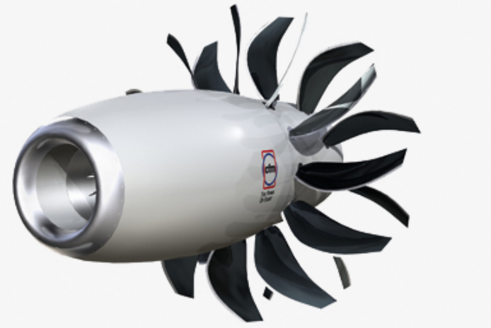
Modern contra-rotating open rotor engine design from CFM (12x10)
