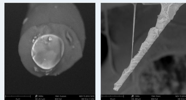
SEM images of the tensile coupon fracture surface show a strong PDMS to glass interface. The role of coupon thickness in the measurement of PDMS and composite breakdown voltage was investigated through fabrication of coupons at various sample thicknesses. Data was plotted based on breakdown voltage measured over a range of sample thicknesses and curve fitted to allow extrapolation to
