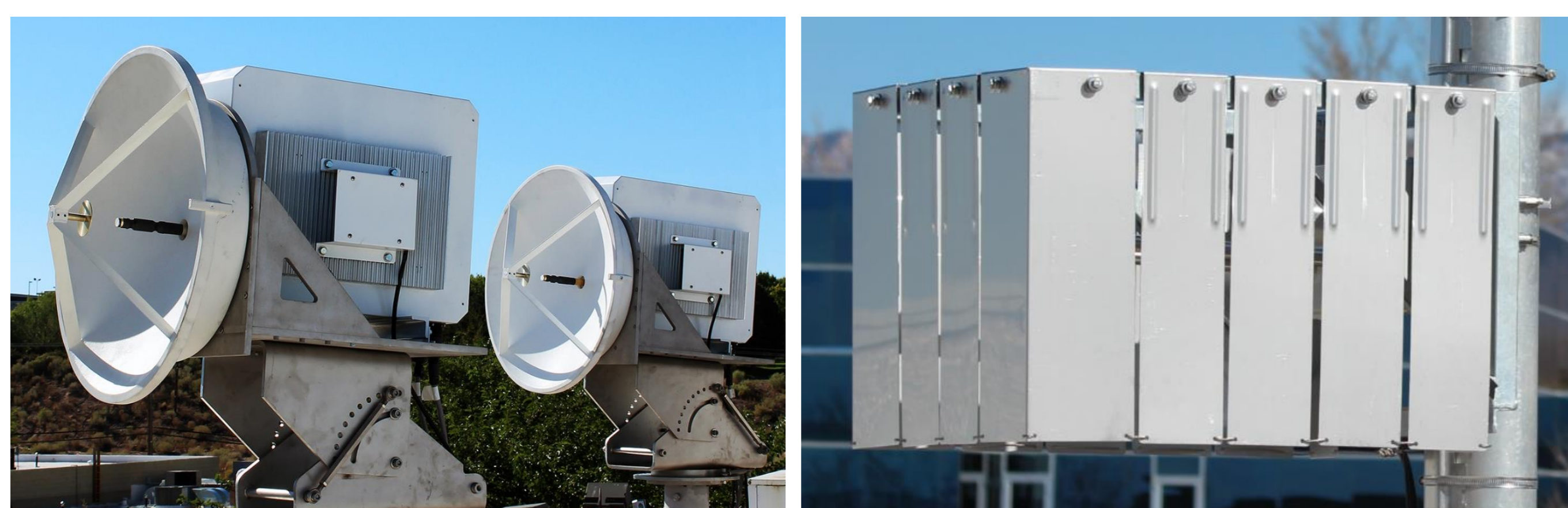
Fig. 2. The twin V/W-band beacon receivers (left) and the Thies Clima optical disdrometer (right).
