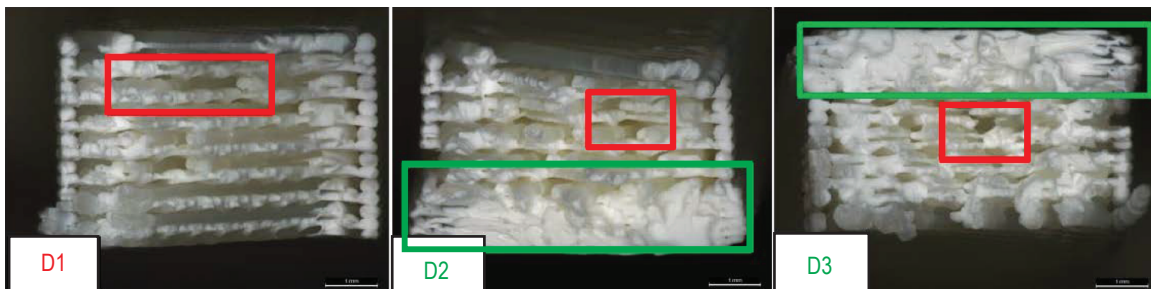
Figure 44. Cross sections of specimens manufactured at the -0.02 mm print head setting. Regions of low and high density are highlighted in red and green, respectively.
