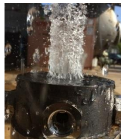
GG-Injector Water Flow Testing
