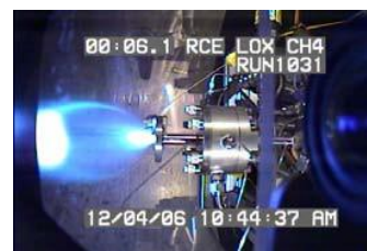
Ascent Main Engine class igniter during vacuum test at GRC
