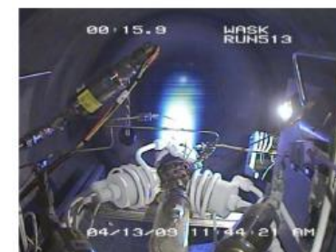
WASK spark-torch igniter during pulse durability testing at GRC
