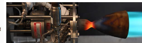
100-lb Aerojet RCE with Unison compact exciter installed at GRC
