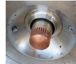
Northrop Grumman Pintle Injector during water tests
