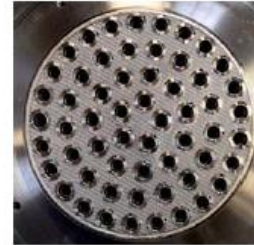
MSFC designed Swirl-Coaxial Injector
