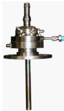
Augmented Spark Impinging (ASI) Igniter developed by MSFC
