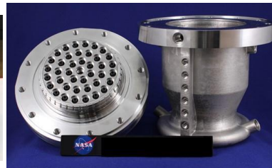
Printed GRCop-84 and printed Inconel Swirl Coax Injector & Chamber
