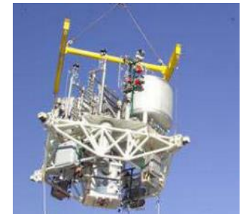
APSTB being installed into WSTF-TS401
