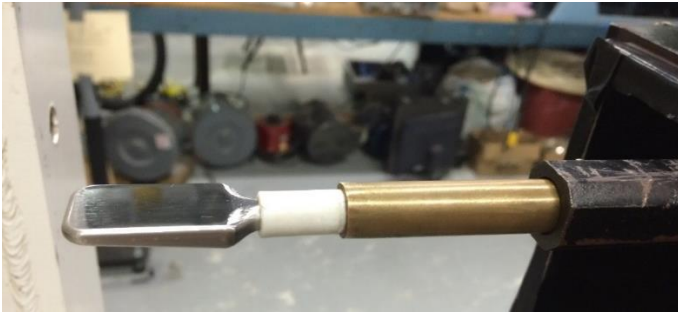
Fig. 6 304 Stainless steel electrode integrated into the wind tunnel sting mount. The white tube is made from polytetrafluoroethylene (PTFE), which is an insulator. The copper tube provides structural support.
