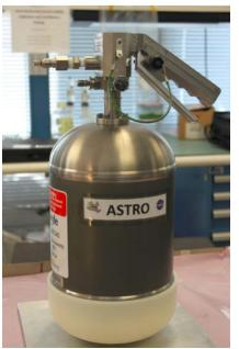
ISS Fine Water Mist Portable Fire Extinguisher Engineering Unit
