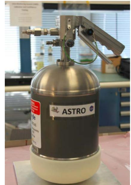
ISS Fine Water Mist Portable Fire Extinguisher Engineering Unit
