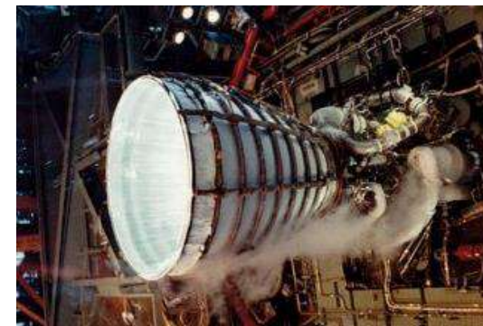
MSFC Space Launch System NASA's RS-25 core stage engine certification testing
