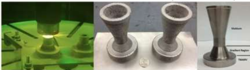
JPL Prototype titanium to niobium gradient rocket nozzle
