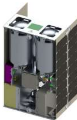
NASA Space Technology Mission Directorate-sponsored Cube Quest challenge for a flight-qualified cubesat (shown: cubesat with an Inconel 718 additively manufactured diffuser section, reaction chamber, and nozzle)
