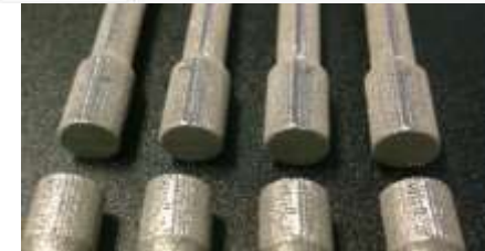
Ti-6Al-4V ASTM E8 compliant dogbones for in situ OM/IR and post-process profilometry, CT and PCRT
