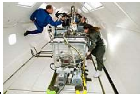
LaRC EBF 3 wire-fed system during parabolic flight testing
