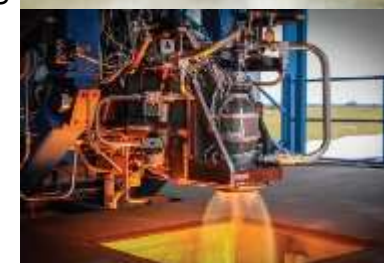
Commercial Crew Program SpaceX SuperDraco combustion chamber for Dragon V2
