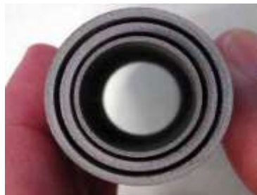
GSFC Reentrant Ti6-4 tube for a cryogenic thermal switch for the ASTRO-H Adiabatic Demagnetization Refrigerator
