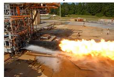
Dynetics/Aerojet Rocketdyne F-1B gas generator injector
