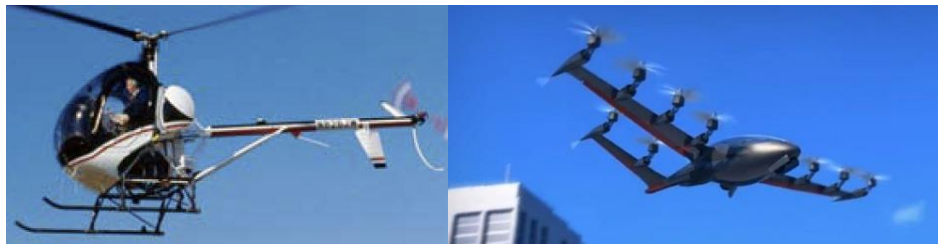
Figure 1. Notional vehicle representations: left) Single Main Rotor (SMR) Helicopter, right) All-Electric VTOL Aircraft.
