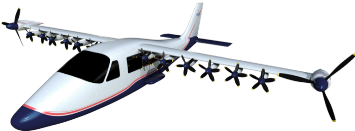
Figure 2. The X-57 Maxwell DEP aircraft. The Tecnam P2006T fuselage and tail with the DEP wing system that includes the wingtip propellers and the high-lift motors.
