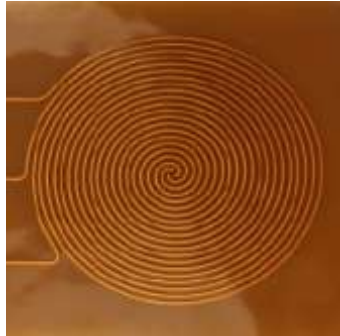
Fig 1. Particle removal system consisting of three parallel spiral-shape conductors designed at ESPL
