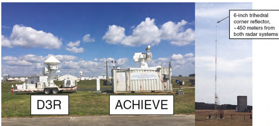
Figure 2.22: Collocated D3R and ACHIEVE radar systems (left), and 30-m calibration tower at WFF (right).
