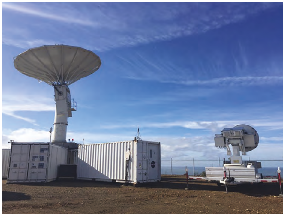
Figure 2.20: NPOL (left) and D3R (right) radars shown deployed along the coast Pacific Ocean near Moclips, Washington. Both radars operated nominally and provided high-quality, multi-frequency (S-, Ka-, and Ku-band) observations of rain, mixed-phase, and ice (snow) precipitation.
