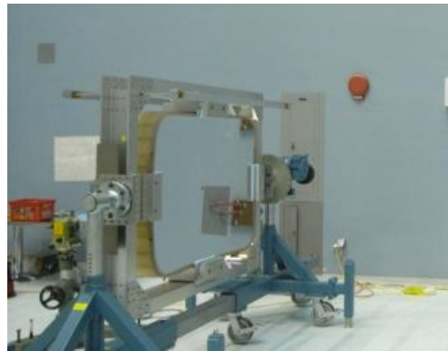
Figure 2 The rectangular 1.4 m x 1 m GSE, spherical, mirror used in proof-of-concept study using an LR to measure the RoC 5 .
