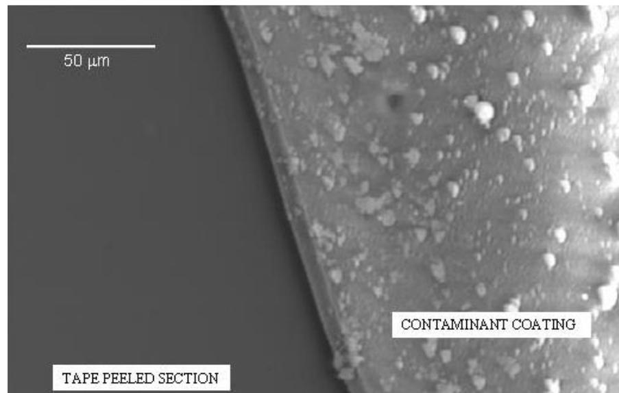
~ 4.6 micron thick silica deposits
