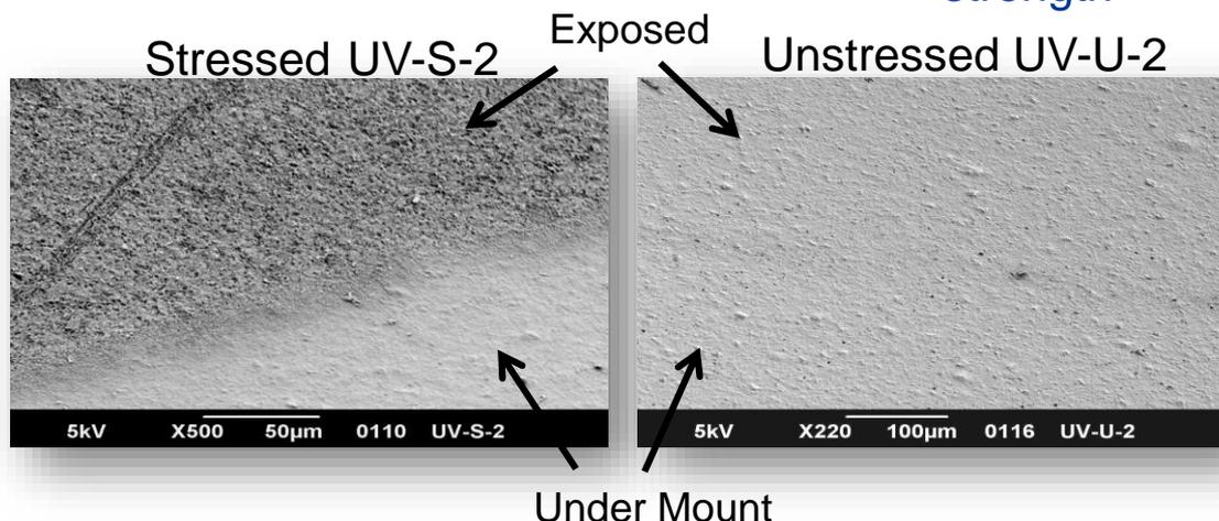
Kapton XC experienced a factor of 4 higher erosion rate under tension
