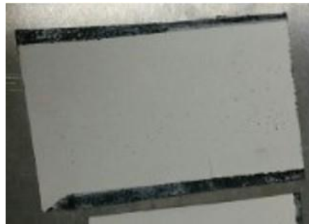
Figure 11. AZ-2000-IECW Painted Black Kapton/Kevlar/Kapton Sample After 75 TVAC Cycles and Tape Lift.
