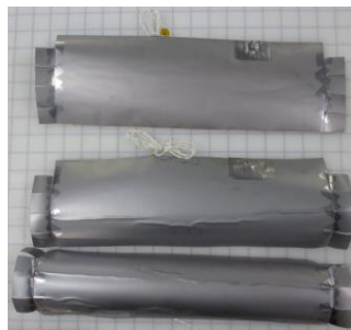
Figure 16. Two Flight and One Spare Flight Kevlar/Polyimide Shells with StaMet Black Kapton for Pigtails.
