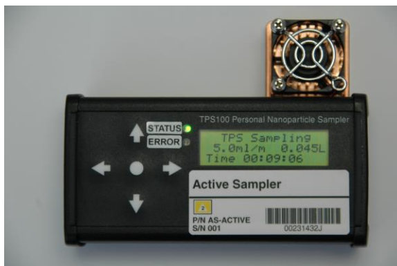
Figure 2. The Active Aerosol Sampler is the modified COTS TPS100™ Personal Nanoparticle Sampler. Commercialized by RJ Lee Group.
