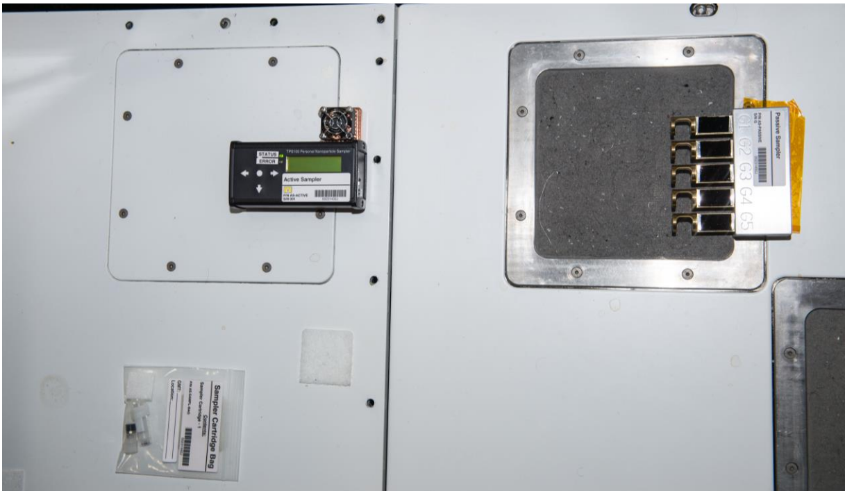
Figure 6. Active and Passive Samplers deployed in Node 3. The Sampler Cartridge Bag is attached to the wall with Velcro nearby and holds the Active Sampler plug and the handle of the cover of the cartridge in use.
