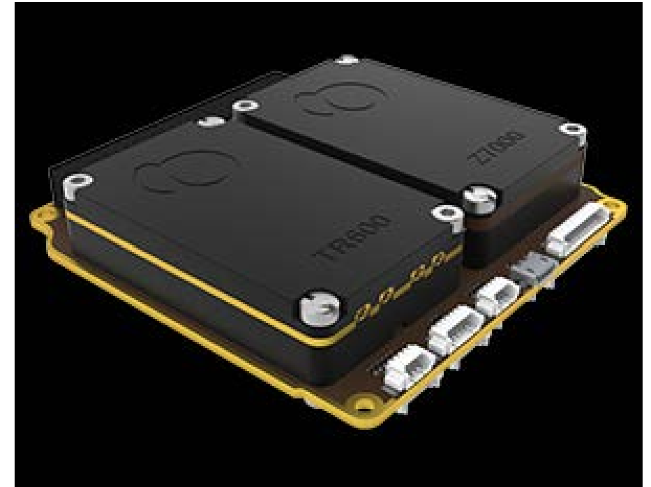
Gomspace FPGA-Based Software Defined Radio
