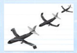
SAW – (Spanwise Adaptive Wing) PI: Matthew Moholt (AFRC) and Co-PI: Dr. Othmane Benafan (GRC): Enabling reconfigurable aircraft through The Spanwise Adaptive Wing (SAW) Concept. Increasing aircraft efficiency by reducing the rudder through the incorporation of SAW. Articulating the outboard portions of the wing via Shape Memory actuation. Lateral-directional stability and control augmentation. Supersonic - Increased compression lift and reduced wave drag for supersonic flying wing design.
