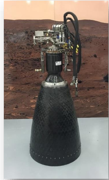
Figure 18: 2,800 lbf thrust JSC2kb-Vac Engine
