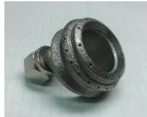
Figure 23. Tank Chill Spray Injector
