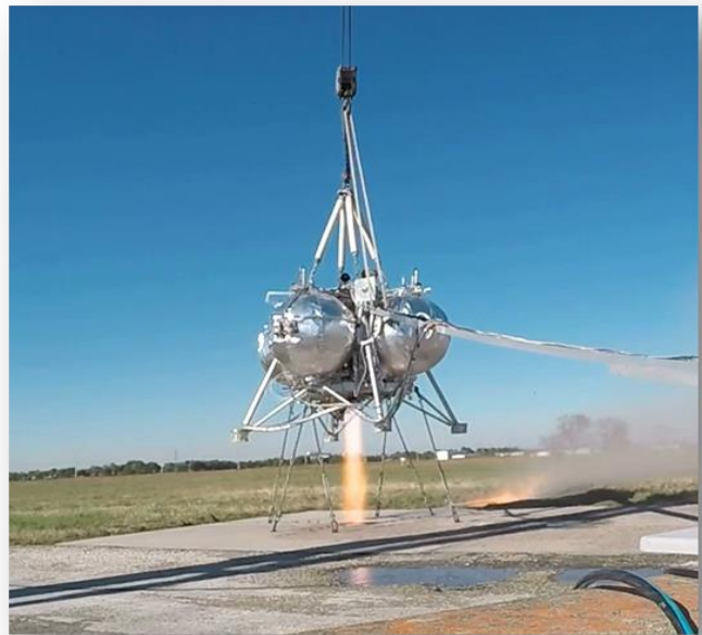
Figure 3. System checkout hot-fire test of the ICPTA at NASA Johnson Space Center
