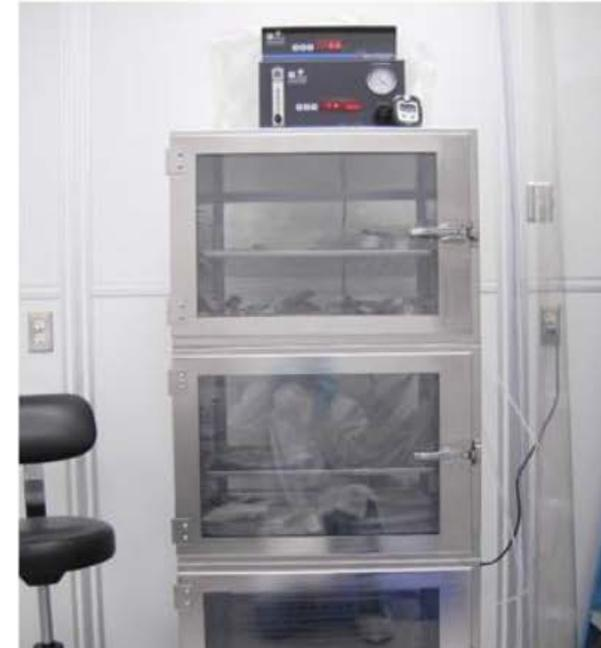
Cabinets identical to the one that houses OSIRIS-REx CK samples have been acquired for Mars 2020 CK samples
