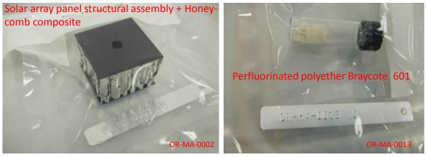
Materials Coupons – Examples of materials used in the spacecraft that are possible sources of contamination.
